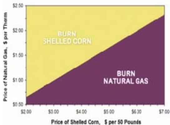
The lines intersect in the “Burn Shelled Corn” portion of the graph. On the basis of heat of combustion, it is cheaper to burn corn than natural gas. However, one must also consider the additional expenses in burning corn versus natural gas such as burner purchase, handling and storage of corn, emissions control, disposal of ash, etc.
